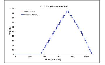
Figure 8. Kinetic of the partial pressure of acetone measured using the SoS Sensor during a DVS experiment
