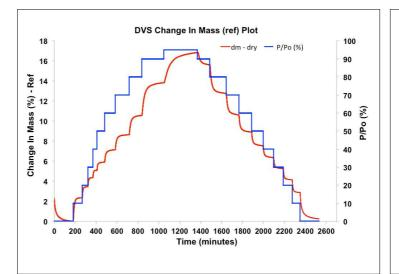
Figure 2. Water sorption kinetics of cellulose membrane at 25 °C
