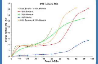
and hexane for a titanium oxide sample at 25 °C
